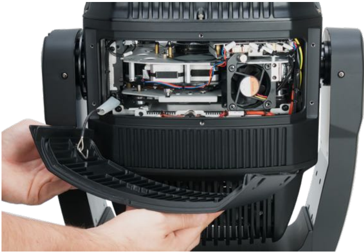
4. Unclip the panel safety cable on one side of the head.
