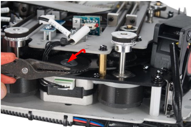
10. Carefully lift the GOBO Holder up and out from the GOBO wheel using small needle nose pliers.
