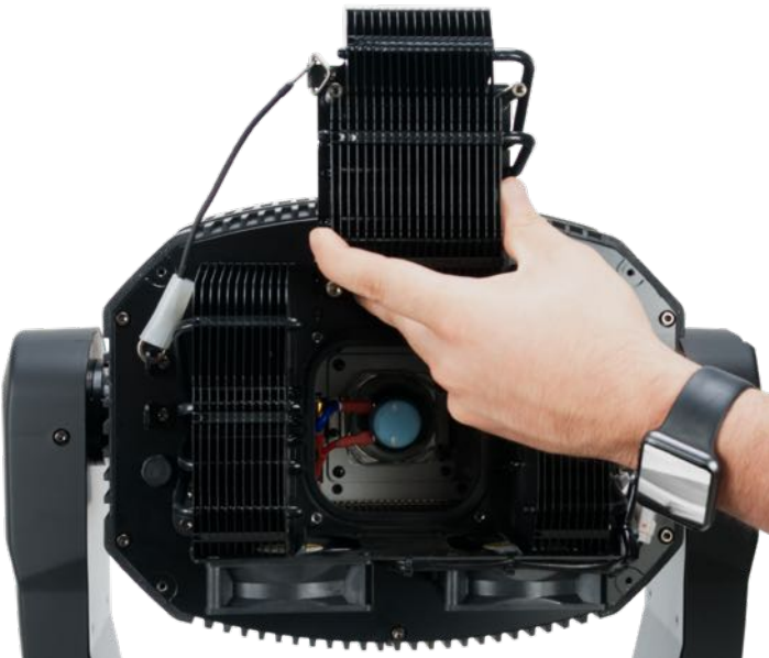
6. Unclip the center heatsink module safety cable.
