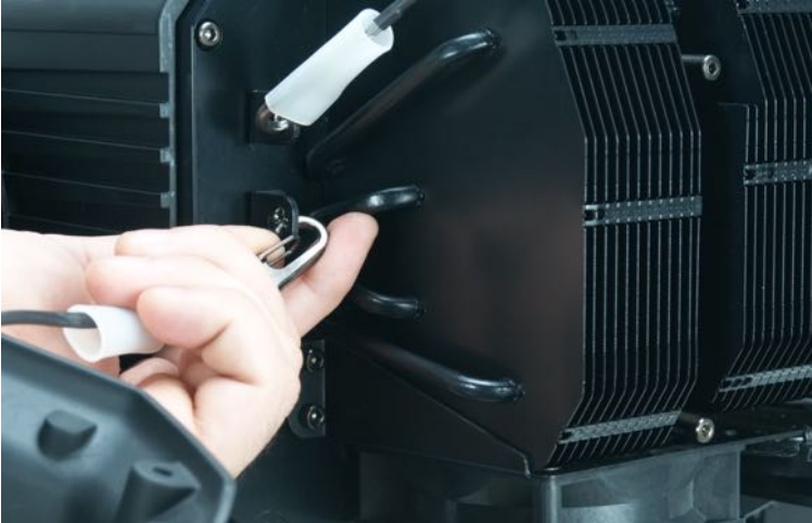
4. Unclip the rear cover safety cable.
